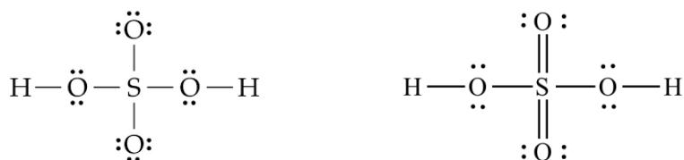
Note that the valence shell of sulfur has an expanded valence, which is permitted for elements below period 2.
