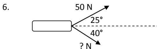
What force is required on the lower rope so that the object travels in a straight line? What is the magnitude of the resultant force?
