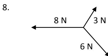
Three forces act on an object. If the object remains in a state of equilibrium, calculate the angle between the lines of action of the smaller forces.
